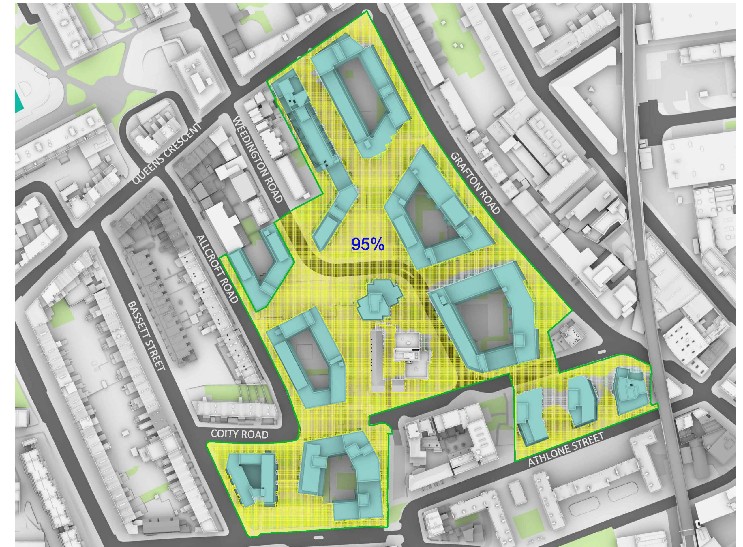
Illustrative Masterplan. Public Realm Sunlight Hours on the Ground on June 21st
