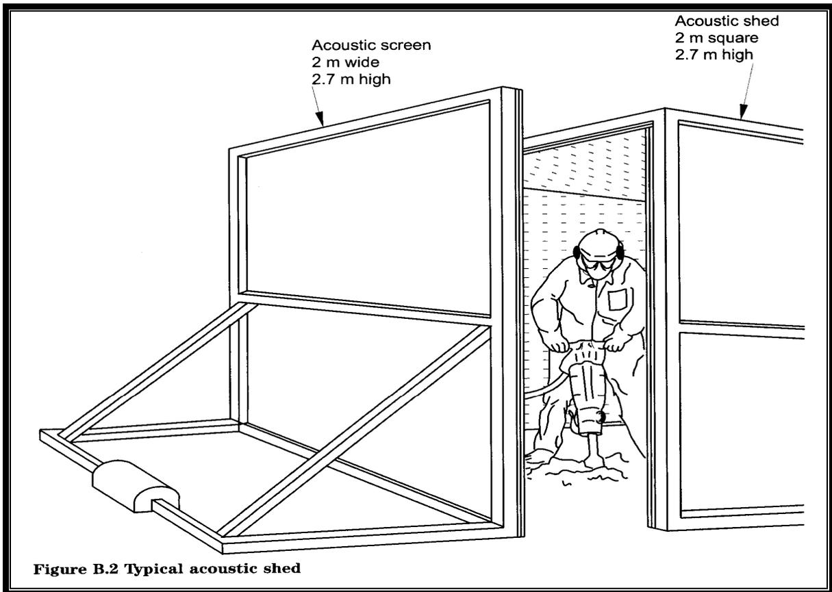
**Figure 4.1b: Typical enclosures to reduce noise nuisance**
