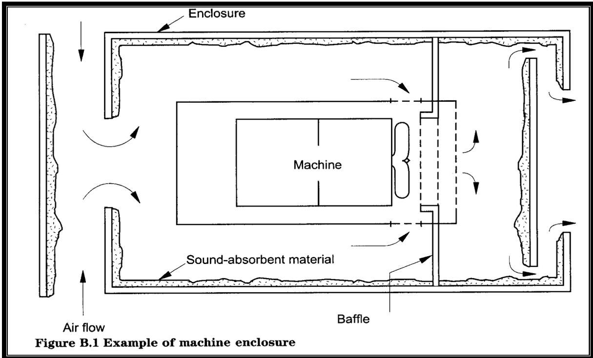
**Figure 4.1a: Typical enclosures to reduce noise nuisance**
